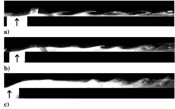
Fig. 2 Flow visualization for Re_{\theta_0} = 107 : a) \sigma = 1.9 , b) \sigma = 3.8 , c) \sigma = 7.6 .
